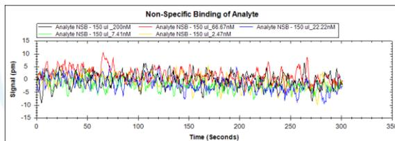
Figure 7. Non-specific binding of analyte to streptavidin coated sensor on OpenSPR
