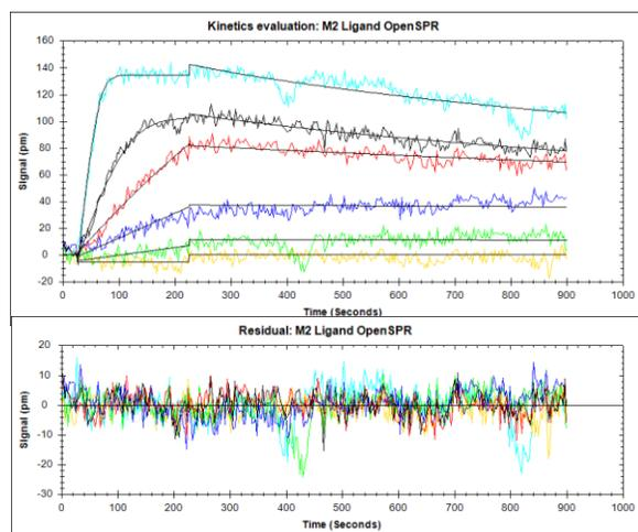
Figure 2. Binding curves and kinetic analysis of M2 ligand on OpenSPR
